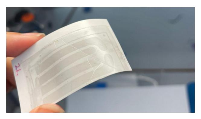
This graphene electronic device rests on temporary tattoo paper and can be transferred to body tissues. A smaller version, tested in rats, can act like a pacemaker.
