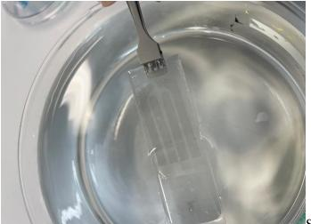
Scientists used an atomically thin layer of graphene in this electronic "tattoo," shown here in water, rendering it highly transparent. Ning Liu/University of Texas at Austin
